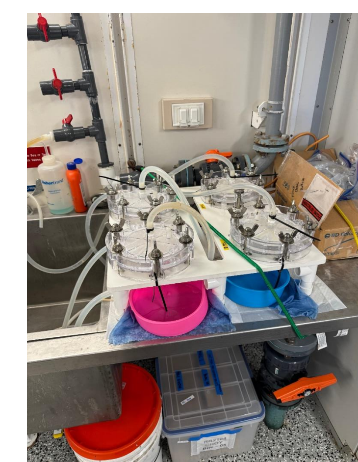
Figure 5. Filtering manifold fabricated and operated by Paul Wojtal on SR2323.
