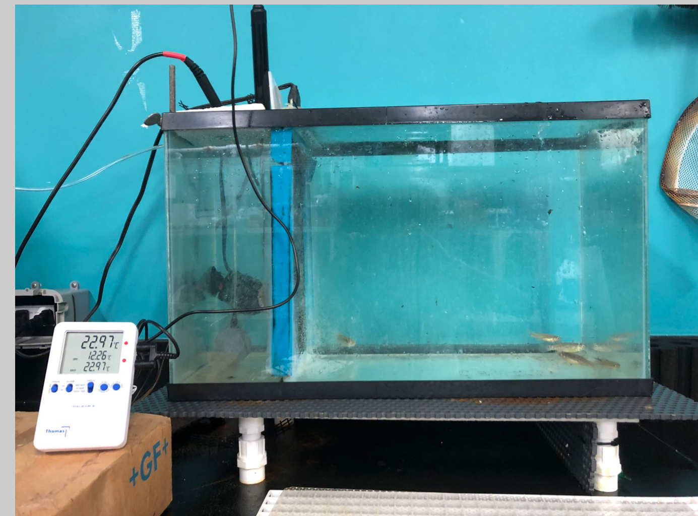
Figure 1. Critical Thermal Maximum set up using F. heteroclitus as the model organism.
