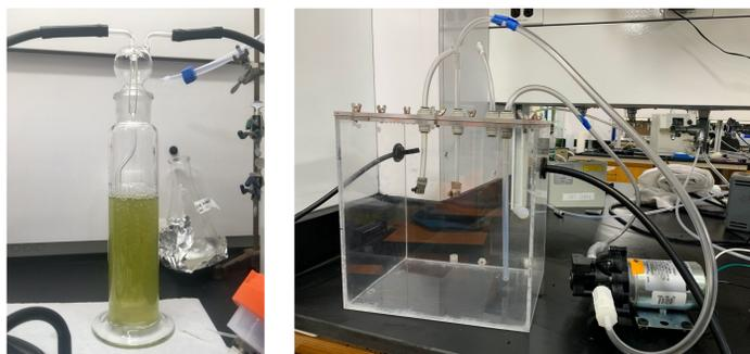
**Figure 3.** Left: Glass frit bubbler with HAB water. Right: Plunging-jet bubbler, pictured with the water pump and two out of three inlets attached. This design is similar to that of May et al. 2016 used for lake spray aerosol
