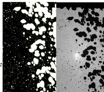
**Figure 5.** Left: The processed image with recognized bubbles outlines in green. Right: The original image from the experiment using the shadowgraph.
